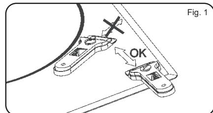
**!** Use only the spatula blade on the ceramic surface avoiding its body coming into contact with the surface as it may scratch it.
