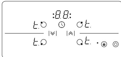
Once the temperature has dropped, the “t” in the heater display will disappear and the hob control unit will revert back into S-Mode. This means that the user can reactivate the appliance by pressing ⓧ.
