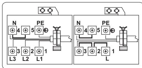
A supply cable  $3 \times 2.5 \text{ mm}^2$ , HO5V V-F, must be used. The ground wire must be connected to the screw marked with the symbol .
